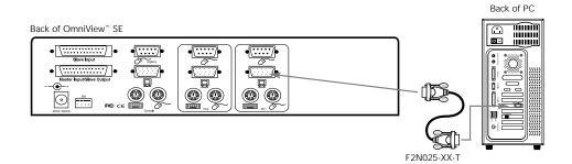
6. Connect the first computer's mouse cable to the OmniView™ SE. If using a PS/2 cable (Belkin Part# F2N036-XX), connect one end to the PS/2 mouse port on the computer, and the other end to the PC1 PS/2 mouse port on the back of the OmniView™ SE. If using a serial mouse cable (Belkin Part# F2N209-XX-T), connect one end to a DB9 serial port on the computer, and the other end to the PC1 DB9 serial mouse port on the back of the OmniView™ SE.
